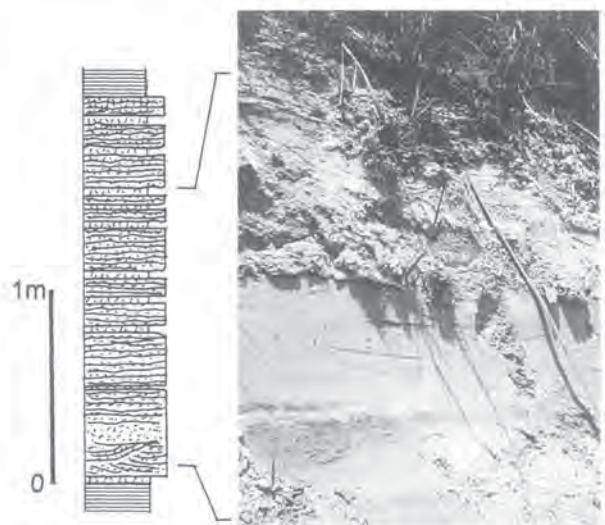
Fig. 9 Geological columnar section and photograph of the Higashihirao volcanic ash bed at Higashihirao (Loc. 6). The facies legends are shown in Fig. 8.
