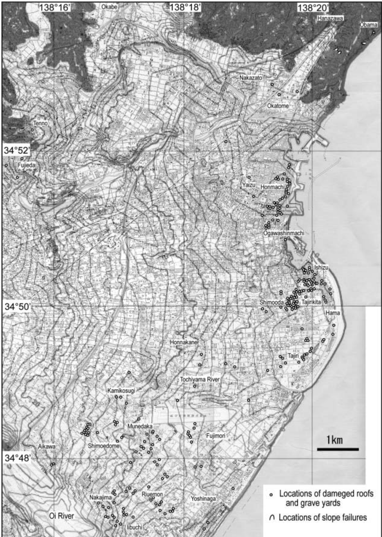
Fig. 6 Damage distribution in Yaizu City. The base map is used the 1/25,000 geographical map of Yaizu and Sumiyoshi published by Geographical Survey Institute of Japan. Contour lines are drawn by 1m under 50m high and 10m over 50m, and from the Digital Map 10m Grid (Elevation) of Yaizu, Sumiyoshi, Shimada and Mukuya published by Geographical Survey Institute of Japan.
